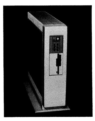
The microPDP-11/53 is typical of the downscaling that has occurred in the PDP-11 Family: the conventional minicomputers that used to comprise the product line have been repackaged as low-end multiuser microcomputers.
