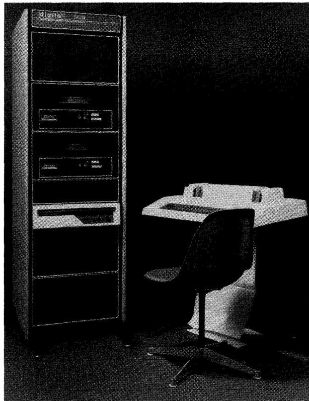
*techniques and are the models after which future PDP-11's will be patterned. The PDP-11/04 basic system with 32K bytes of MOS memory is priced at \$7,695. The 11T34 packaged system includes an 11/34 CPU with 64K bytes of core or MOS memory, dual RK05 2.4-megabyte disk drives (4.8 megabytes total), and an LA36 DECwriter II console and sells for \$30,900. Monthly maintenance charge for the 11T34 system is \$263.*
