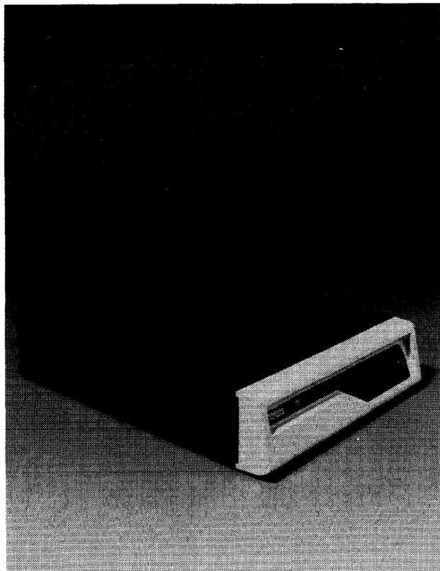
*The heirs-apparent to the PDP-11 line are the PDP-11/04 (left) and the PDP-11/34, shown at right in a standard package configuration, the PDP-11T34 system. The two computers use the same backplane and memories. The only difference between them is in memory management hardware, present on the PDP-11/34 and not included in the PDP-11/04. The 11/04 can have up to 56K bytes of memory, while the 11/34 can address up to 248K bytes. These newest PDP-11's use more cost-effective packaging*
