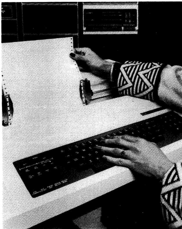
*The PDP-11/70 represents the high end of one of the most extensive minicomputer product lines in existence today. In the foreground is the LA37 DECwriter II terminal, one of the numerous terminals now offered with the PDP-11 processors. The PDP-11/70 is a high-performance machine with integral cache memory and high-speed 32-bit data paths. The system also has memory management, look-ahead, and internal memory expansion capability up to 2048K bytes.*
