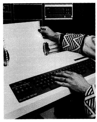
The PDP-11/70 represents the high end of one of the most extensive minicomputer product lines in existence today. In the foreground is the LA37 DECwriter II terminal, one of the numerous terminals now offered with the PDP-11 processors. The PDP-11/70 is a high-performance machine with integral cache memory and high-speed 32-bit data paths. The system also has memory management, lookahead, and internal memory expansion capability up to 4096K bytes.
