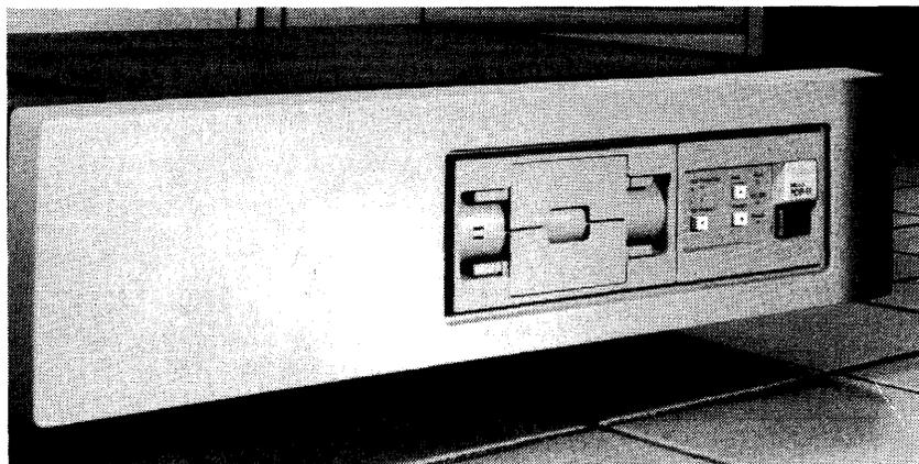
*The Micro/PDP-11 is the low-end system in DEC's PDP-11 family. Based on the PDP-11/23-PLUS CPU, the Micro/PDP-11 supports from 256KB to 4MB of main memory and 10MB to 38MB of mass storage. It can also control up to six concurrently active workstations. The Micro/PDP-11 can run such standard PDP-11 operating systems as RT-11, RSTS/E, and V7M-11 Unix, as well as Micro/R SX, a specially extended version of RSX-11M-Plus.*
