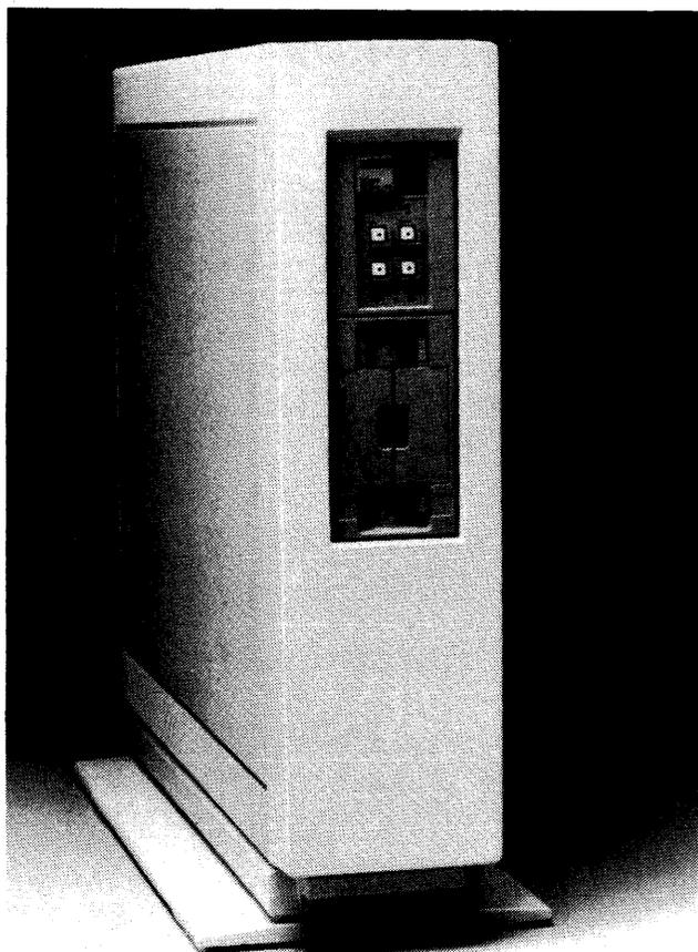
*The MicroPDP-11/73 incorporates DEC's new 15MHz J-11 chip set, and, when fully configured, delivers about 75 percent of the performance of the top-of-the-line PDP-11/44 minicomputer. The MicroPDP-11/73 can support up to 4MB of memory and can accommodate up to 14 workstations, with 4 to 12 concurrently active.*
