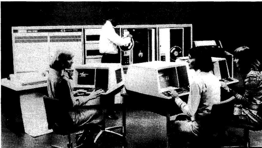
*The VAX-11/780 32-bit computer system supports up to 64 interactive users as well as multi-stream batch processing. The VAX/VMS virtual memory operating system features a full demand-paging operation that allows programs to be as large as 32 megabytes. The 32-bit word length enables the system to support up to 2 million bytes of real, error-correcting MOS memory.*
