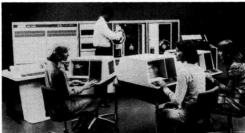
The VAX-11/780 32-bit computer system supports up to 96 interactive users as well as multi-stream batch processing. The VAX/VMS virtual memory operating system features a full demand-paging operation that allows addressing space of up to one billion words. The 32-bit word length system supports up to 2 million words of real, error-correcting MOS memory.
