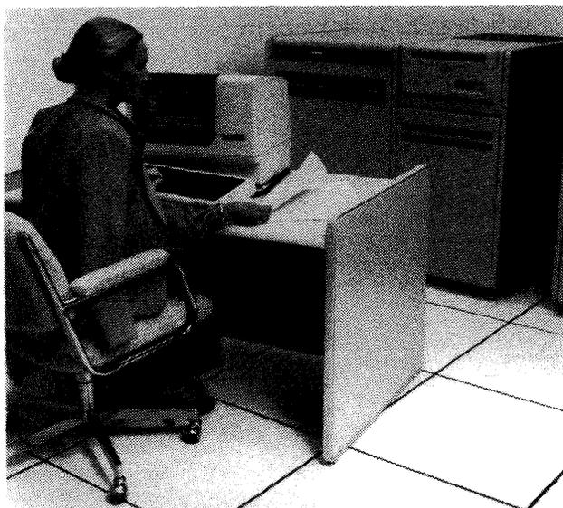
The VAX-11/750 virtual memory computer is a 32-bit system that uses advanced LSI circuit technology to achieve low price and compactness for a wide variety of environments. The entry-level system configuration, with 512K bytes of memory and two 28-million-byte disk drives, is priced at \$89,900.
