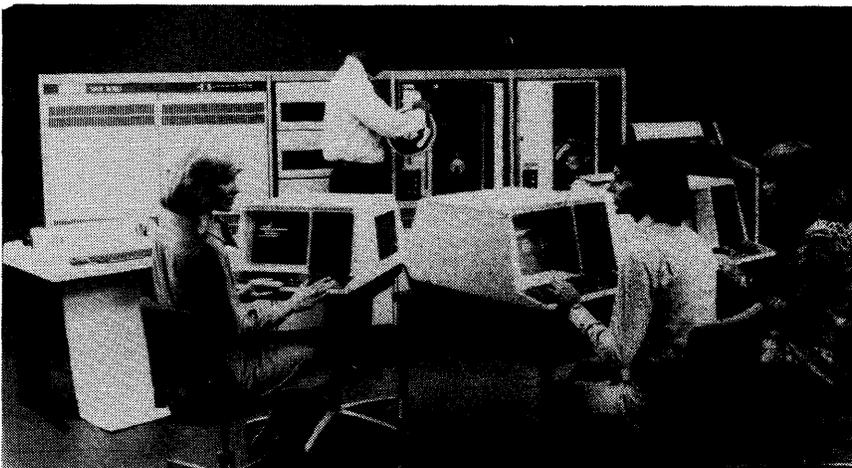
The VAX-11/780 32-bit computer system supports up to 96 interactive users per UNIBUS as well as multi-stream batch processing. The VAX/VMS virtual memory operating system features a full demand-paging operation that allows addressing space of up to one billion words. The 32-bit word length system supports up to 2 million words of real, error-correcting MOS memory.
