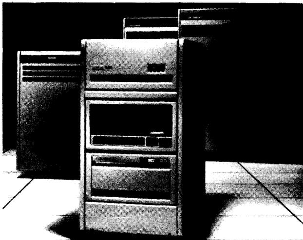
The newest member of Digital Equipment Corporation's VAX family of virtual memory computers is the VAX-11/730, shown above in a single, 42-inch high cabinet with 131 megabytes of fixed and removable disk storage. Other VAX systems pictured are the mid-range VAX-11/750 (left), VAX-11/780 (right), and the VAX-11/782 attached processor system (rear). Prices range from \$48,900 for an entry-level VAX-11/730 package to \$445,000 for the top-of-the-line VAX-11/782 package.
