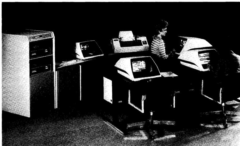
*The PDP-8/E-based DEC Datasystem 340 shown here is operating under the foreground/background multi-programming option that permits simultaneous data entry at any of three terminals concurrent with background batch processing.*
