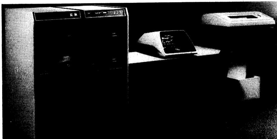
*The PDP-8/E-based DEC Datasystem 340 can operate under a foreground/background multi-user option that permits simultaneous data entry at any of up to seven terminals concurrently with background batch processing. This system complete with operator's CRT, printer, two cartridge disk drives, 9-track tape drive, and COS software costs \$50,680.*
