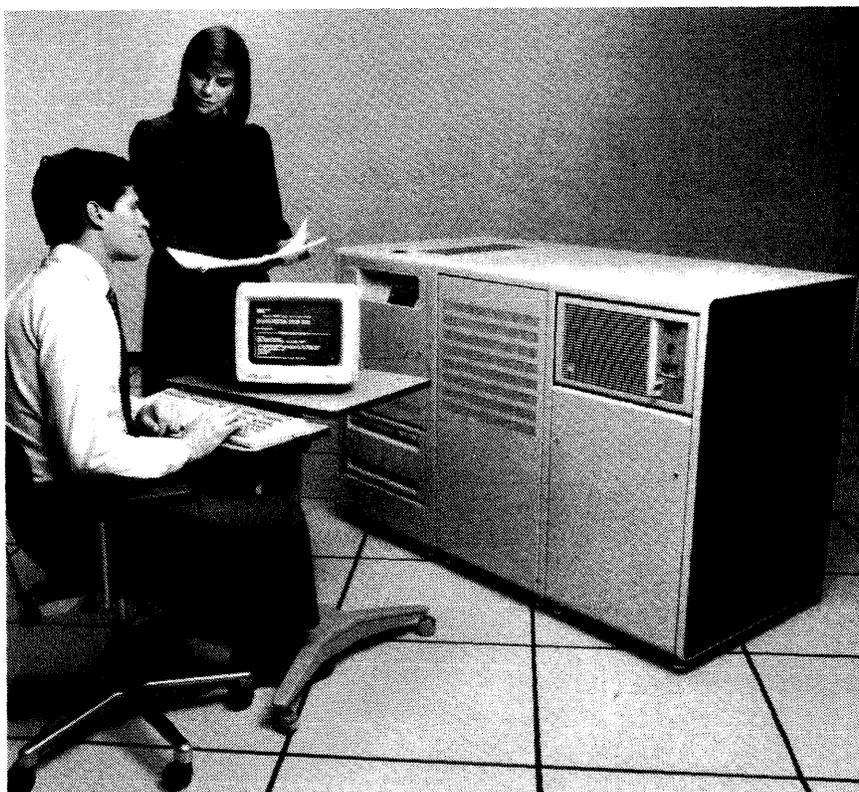
*Digital Equipment Corporation's VAX 8200 is the successor to the widely installed and highly regarded VAX-11/780. Providing the same power as its predecessor, the VAX 8200 is intended as a department-level processor in office automation, commercial, and manufacturing applications.*
