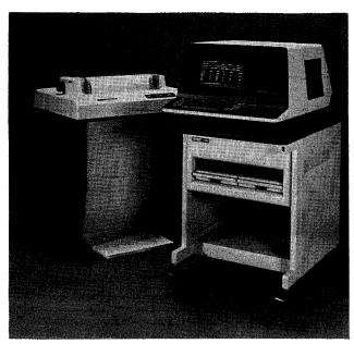
A basic Datasystem 308, consisting of a VT78 video terminal/central processor with 32K bytes of MOS memory and a dual floppy disk system, is shown in the standard mini-desk enclosure, with the optional LA78 printer at left. The basic system purchase price of \$12,600 also includes the COS-310 operating system, DEC's DIBOL business-oriented language, and system installation. The monthly maintenance charge is \$68. The LA78 printer is available for \$3,300.
