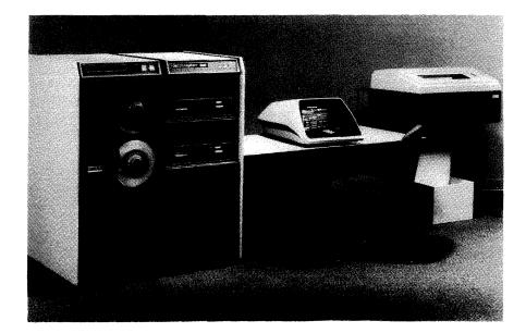
The PDP-8/E-based DEC Datasystem 340 can operate under a foreground/background multi-user option that permits data entry at multiple terminals concurrently with background batch processing. This system, complete with operator's CRT, printer, two cartridge disk drives, 9-track tape drive, and COS software, costs \$54,765.
