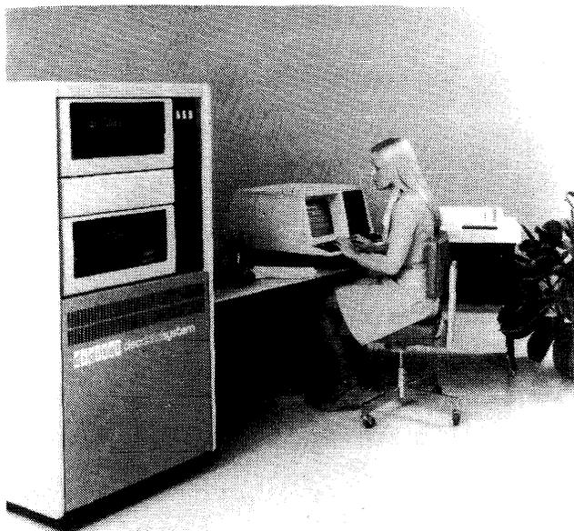
Utilizing the PDP-11/34 processor, this DEC Datasystem 530 offers the advantages of the CTS-500 software and supports a maximum of 32 terminals, 248K bytes of core memory, and up to 1.5 billion bytes of disk storage. Users can grow from the Datasystem 300 family into the Datasystem 530 and 570 systems without worrying about software compatibility, since DIBOL-11 is a standard language on all Datasystems.
