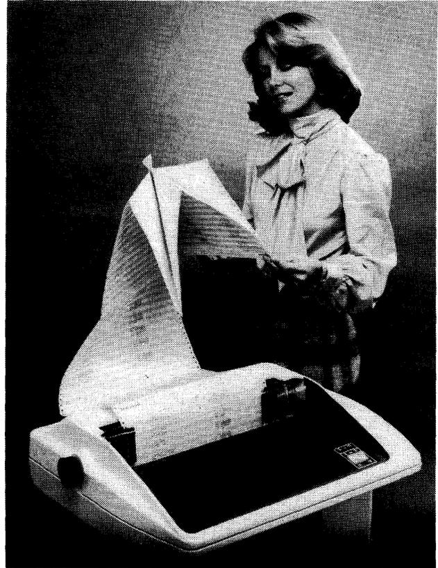
*The Dasher LP2, Data General's first in-house manufactured printer, prints at 180 cps and features bi-directional printing and built-in logic to cause spacing or skipping directly to the next character to be printed. Its dot matrix printing mechanism allows printing at 6 or 8 lines per inch with standard, elongated, compressed, or elongated-compressed character sizes.*
