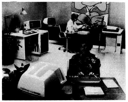
Data General Corporation's Commercial Systems CS/10 is a new lowend computer for companies in the \$100,000 to \$20 million range. The interactive COBOL-based system can expand from a single-station system with 2.4MB of diskette storage to a four display system with up to 50MB of disk storage.
