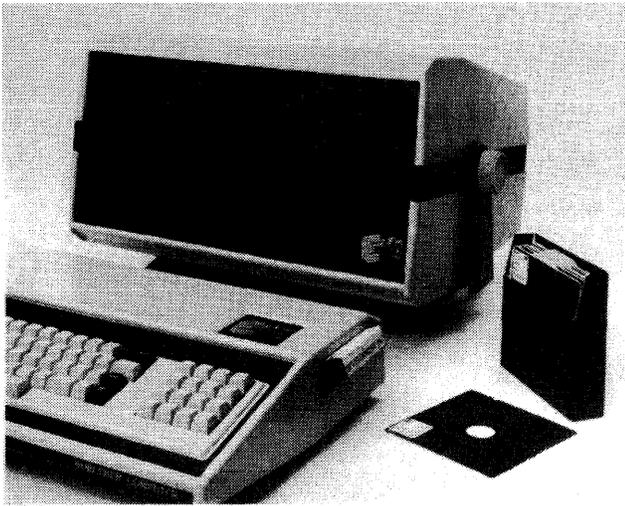
Two of the most novel design aspects of the Sorcerer are illustrated here. A 32KB system is shown with a modified 8-track tape cartridge container housing a ROM Pac inserted in its normal position at the right side of the keyboard chassis. The Composite Video/Disk unit at the rear has a 12-inch B/W screen and contains two 5 1/4-inch floppy disk drives capable of storing more than 600KB of programs and/or data.
