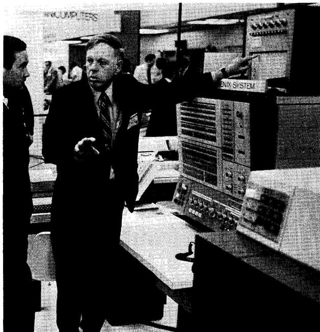
*The Phoenix X-30 console will be comfortably familiar to anyone who has operated an IBM 360/30. Atop the CPU cabinet is a multiple-pen chart recorder that was used to measure and analyze the system's performance on live benchmark tests at the National Computer Conference.*
