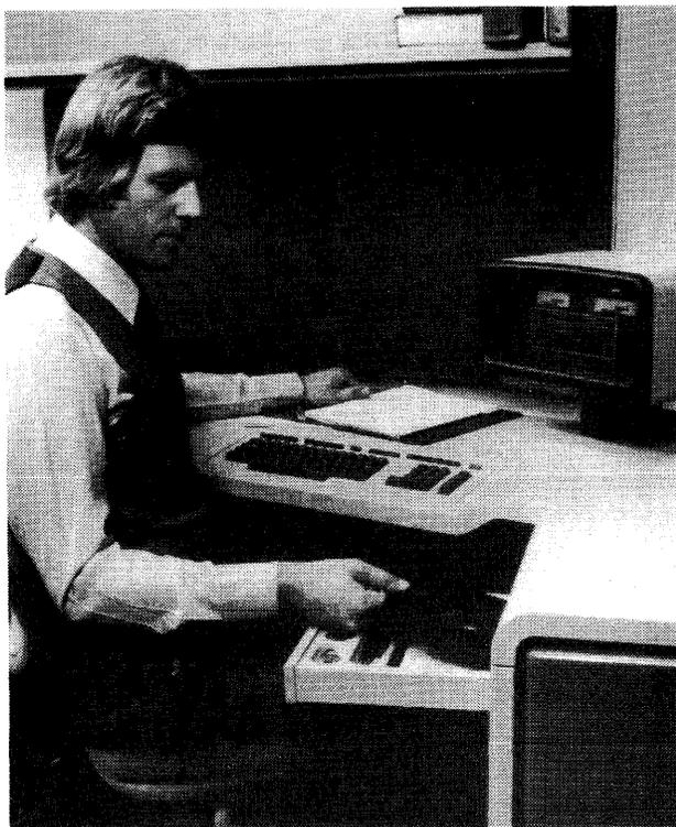
The HP 250 is controlled from a desk-like console with keyboard and a display screen which tilts, swivels, and slides from left to right to virtually any position desired by the operator. Eight programmable "softkeys" below the screen can be used for calling in routines and programs and for communications between the operator and the system.
