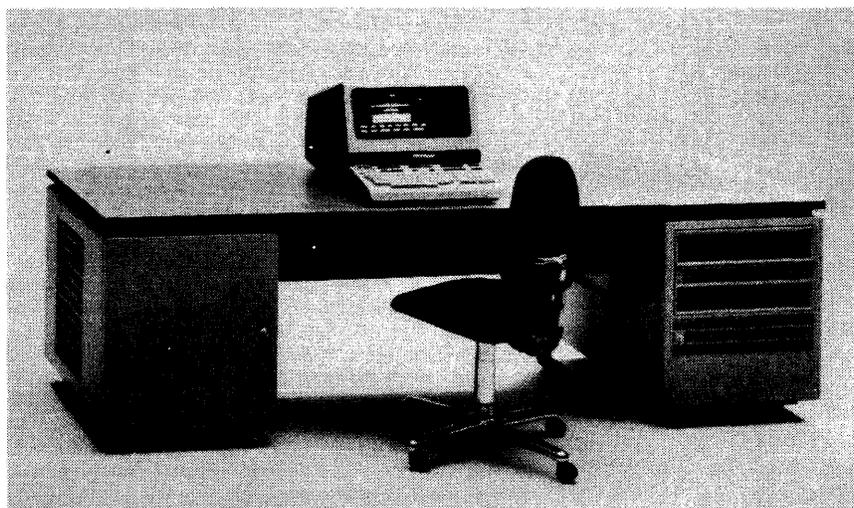
The top of the line among the HP 1000 packaged systems is the Model 45, which combines the new 2117F processor, high-performance RAM memory, the HP 2648A Graphics Terminal, the HP 7906 Disc Subsystem, and the RTE-IV Operating System. The system is expandable to 1280K bytes of memory and supports 10 I/O channels in this desk configuration.
