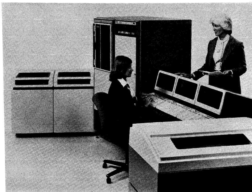
*This large HP 3000 Series III system includes a one-megabyte fault-control memory, two 7925 120-megabyte disk drives, a 7970E 1600-bpi tape drive, a 2617 600-lpm printer, a 2640B console, and two additional 2645A terminals. All of the peripheral equipment is manufactured by Hewlett-Packard.*
