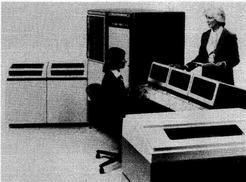
*This large HP 3000 Series III system includes a one-megabyte fault-control memory, two 7925 120-megabyte disk drives, a 7970E 1600-bpi tape drive, a 2617 600-lpm printer, a 2640B console, and two additional 2645A terminals. All of the peripheral equipment is manufactured by Hewlett-Packard.*
