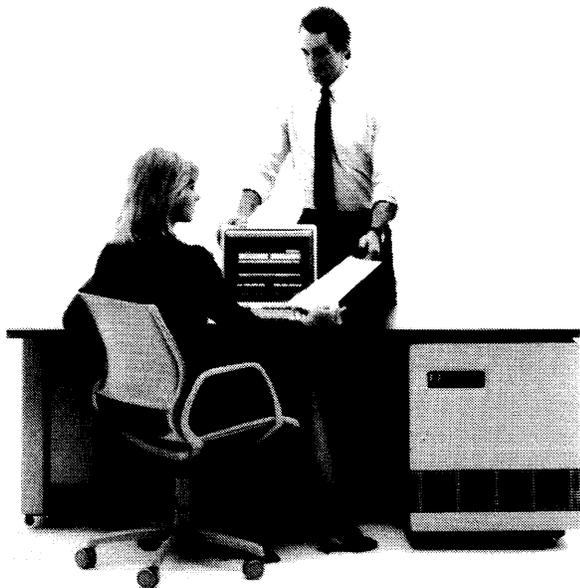
*The Series 58 is the mid-range system in the HP 3000 family, and according to HP, offers 50 percent higher performance than the Series 48. The Series 58 supports up to 152 users, 8MB memory, 32KB cache memory, and 4.2GB storage. Up to eight tape drives are also supported. The Series 58 is fully compatible with all other members of the HP 3000 family.*
