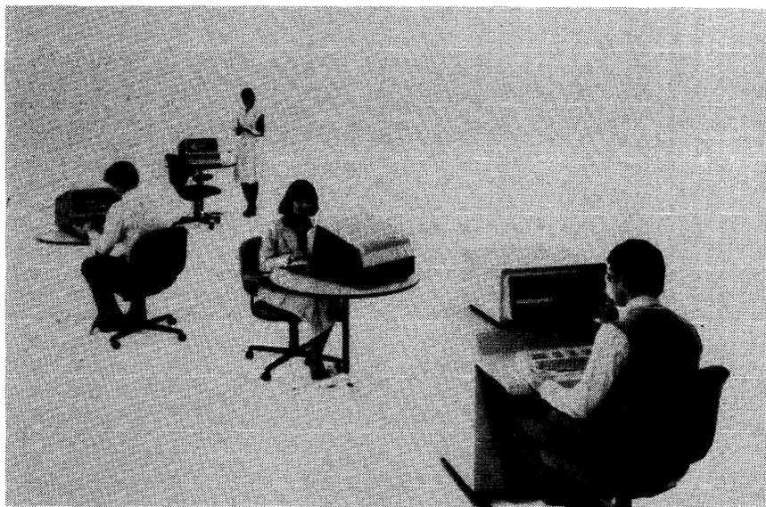
The HP 300 is a general purpose computer that "takes no more space than a free-standing data terminal." The system can support up to 16 terminals, a million bytes of memory within the basic enclosure, and 490 million bytes of external disk storage.
