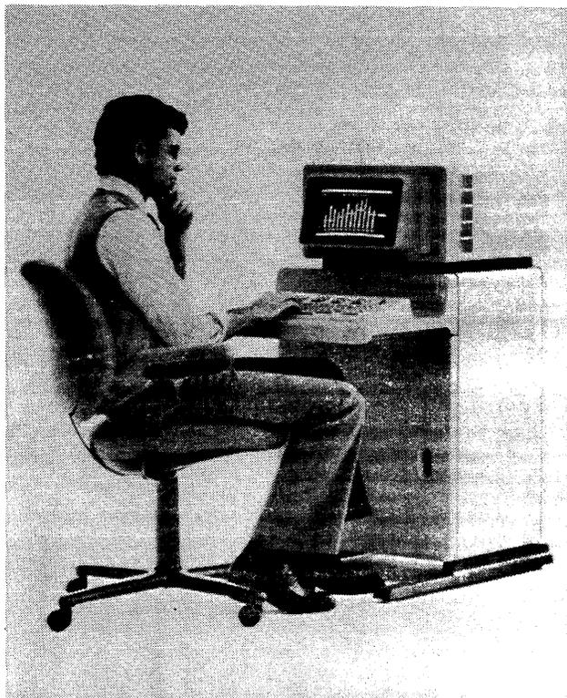
The HP 300 Integrated Display System (IDS) is used to schedule, monitor, and control the concurrent activities of the Amigo/300 operating system. The IDS screen can be split into eight "windows," independently controlled, which can be attached to a data file and scrolled both vertically and horizontally to make entries or changes.
