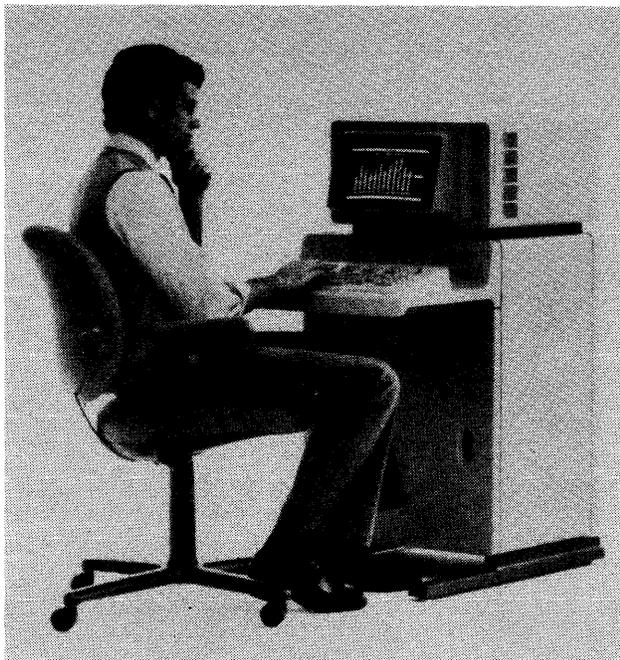
The HP 300 Information Display System (IDS) is used to schedule, monitor, and control the concurrent activities of the Amigo/300 operating system. The IDS screen can be split into eight "windows," independently controlled, which can be attached to a data file and scrolled both vertically and horizontally to make entries or changes.
