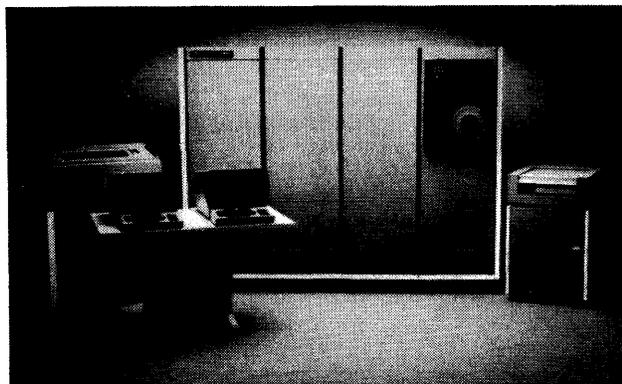
The Harris 800 system above includes (left to right) a Model 4130 900-lpm printer, an operator console and MAP terminals, the H800 CPU with memory and I/O expansion cabinets, a Model 6890 nine-track magnetic tape drive, and a Model 5650 300-megabyte disk storage module.
