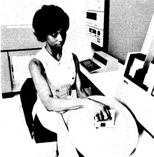
*A drawer beneath the 5424 Multi-Function Card Unit houses the compact 5444 Disk Storage Drive and its removable single-disk cartridge.*
