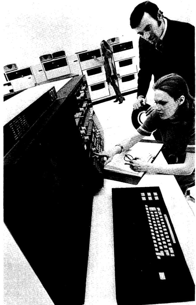
*The System Console of the new Model 168 system features a CRT display and keyboard. In the background is a 3330 Disk Storage facility, which stores 100 million bytes per spindle.*
