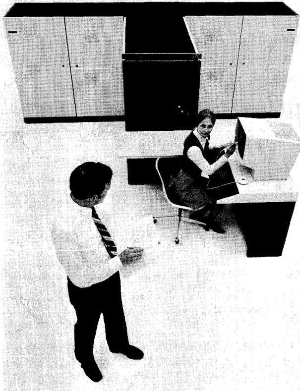
*The System/370 Model 158 Processing Unit, introduced in August 1972, provides up to 2 million characters of MOS main storage and up to 16 million characters of virtual storage. A feature of the Model 158 is its CRT display console with light-pen input.*
