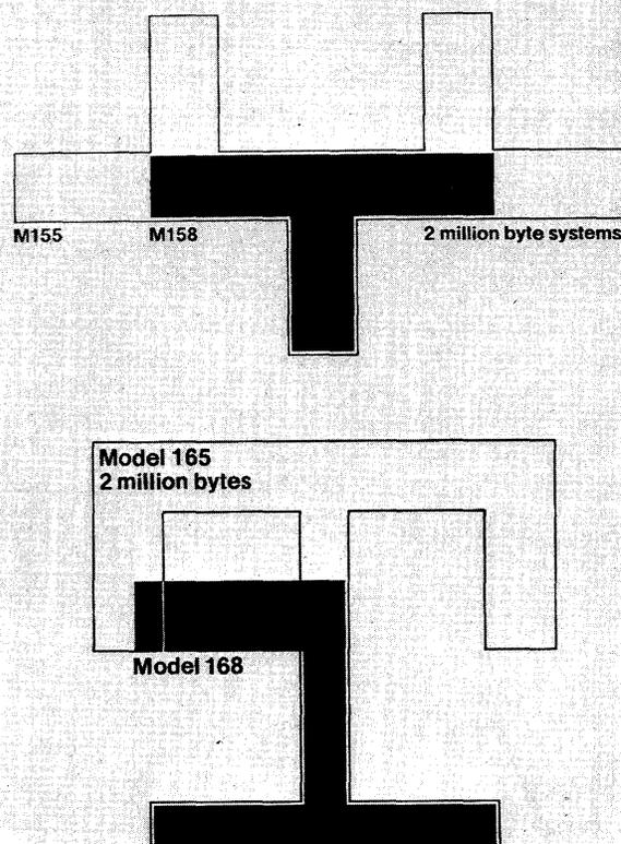
IBM's new MOS main memories result in greatly reduced floor-space requirements. The top illustration shows a 2-million-byte Model 158 CPU (shaded black) superimposed against a Model 155 with the same amount of core storage. Below, a 2-million-byte Model 168 CPU is similarly compared with a Model 165 of equivalent capacity.
