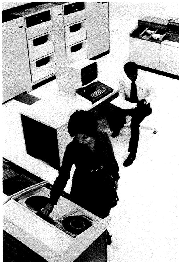
High-speed peripheral equipment for the Model 125 is currently limited to the 3330 Series Disk Storage drives (left rear), which provide up to 400 million bytes of on-line storage, and the 3410/3411 Magnetic Tape Units (left foreground), which provide data rates of up to 80,000 bytes/second.
