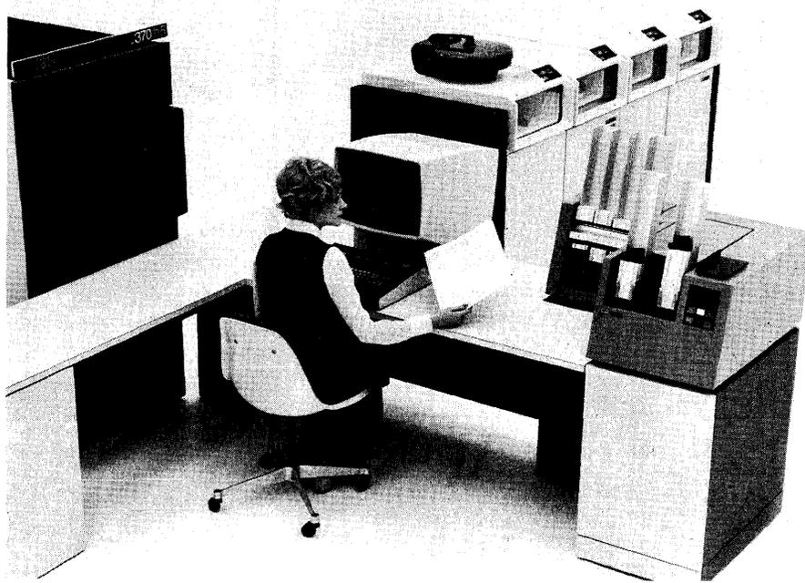
*The Model 115, the smallest and newest member of the expanding System/370 family, employs distributed processing techniques and features integrated control units for attachment of disk drives, magnetic tape units, card unit, line printer, and communications terminals.*
