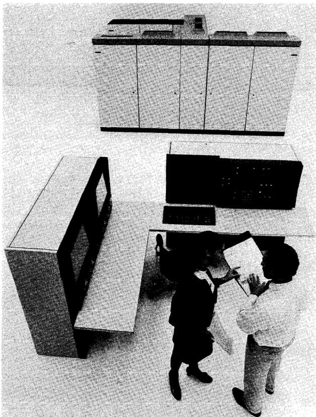
*The Model 168, largest of IBM's virtual-storage computers, offers up to 8 million bytes of real MOS main storage; a dual-processor 168 MP system can have up to 16 million bytes. The Model 168 console features a CRT display and keyboard.*
