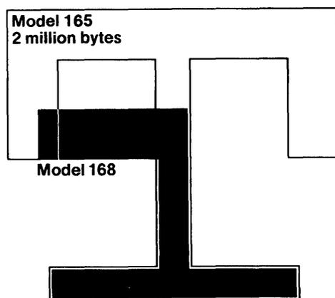
IBM's new MOS main memories result in greatly reduced floor space requirements. The top illustration shows a 2-million-byte Model 158 CPU (shaded black) superimposed against a Model 155 with the same amount of core storage. Below, a 2-million-byte Model 168 CPU is similarly compared with a Model 165 of equivalent capacity.
