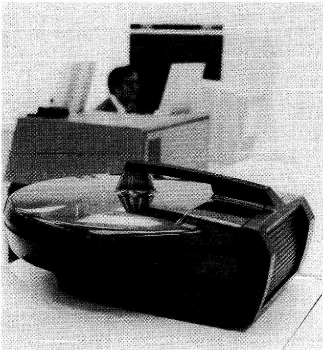
The 3348 Data Module, used in IBM's 3340 "Winchester" Direct Access Storage Facility, stores up to 35 million or 70 million bytes of data and combines the disks, access arms, and read/write heads into a single sealed cartridge.
