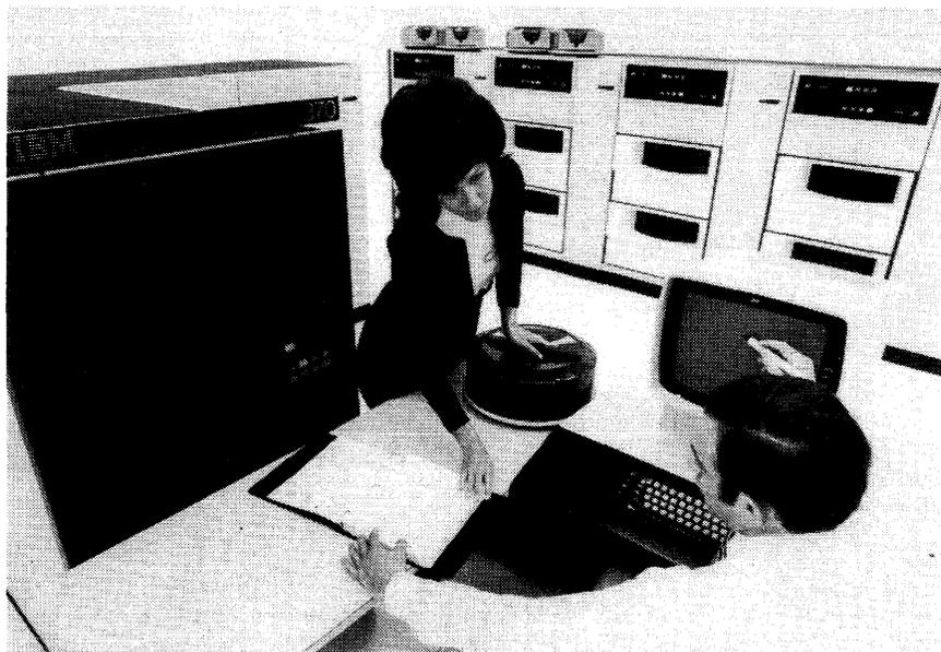
*The Model 158 Processing Unit provides up to 4 million bytes of MOS main storage and is available in both uniprocessor and dual-processor (MP) configurations. A feature of the Model 158 is its CRT display console with light-pen input. An 8-drive 3330 Disk Storage subsystem is in the background.*
