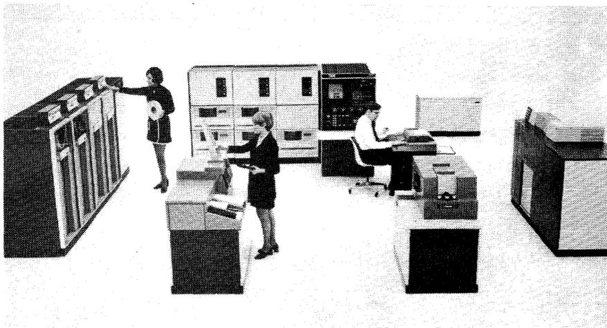
*This Model 135 configuration includes a 5-drive disk storage subsystem attached directly to the central processing unit at center rear. In the foreground, from left to right, are the 3803/3420 Magnetic Tape Subsystem, 3505 Card Reader, 3525 Card Punch, and 3211 Printer.*
