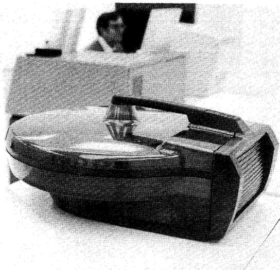
*The 3348 Data Module, used in IBM's 3340 "Winchester" Direct Access Storage Facility, stores up to 35 million or 70 million bytes of data and combines the disks, access arms, and read/write heads into a single sealed cartridge.*
