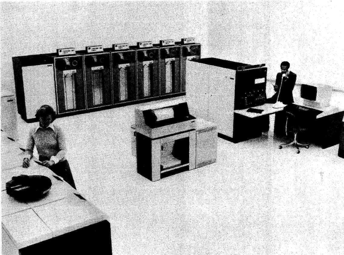
The Model 138 is one of the two System/370 processor models still in new limited production at this writing.
