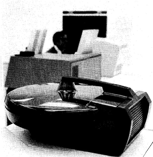
*Weighing in at 16 or 18 pounds, the two models of IBM's new 3348 Data Module store up to 35 million or 70 million bytes of data, respectively, and combine the disks, access arms, and read/write heads into a single sealed cartridge.*
