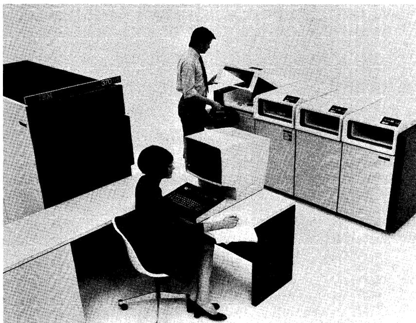
*The Model 115, like the architecturally similar Model 125, includes a standard operator console with CRT display. The operator in the background is mounting a 3348 Data Module on a 3340 Disk Storage drive.*
