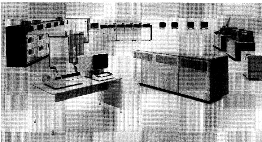
*The 4341 processor provides 2 to 16 megabytes of main memory, 4K to 16K bytes of buffer storage, and up to 6 I/O channels. It can utilize virtually all of the System/370 communications and peripheral equipment, including the high-performance 3380 Direct Access Storage Device. The 4341 supports the MVS operating system as well as OS/VSI, VM/370, and DOS/VSE.*
