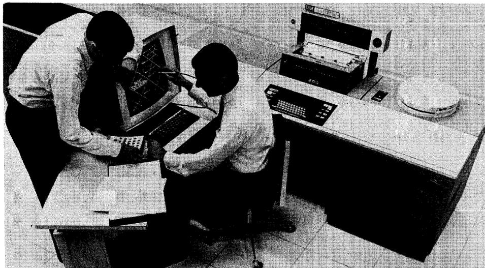
*This IBM 1130 configuration centers on the 2250 graphic display unit with light pen input. Also shown are a cartridge for the integral single-disk drive, and the console with keyboard and printer.*
