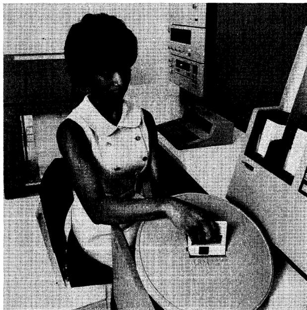
*In the System/3 Model 10, the compact 5444 Disk Storage Drive and its removable single-disk cartridge are conveniently housed in a drawer beneath the 5424 Multi-Function Card Unit.*
