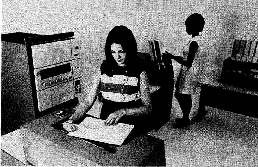
*This view of a System/3 Model 10 installation shows the CPU at left, the 5203 printer in the foreground, the 5424 Multi-Function Card Unit at center rear, and the off-line 5486 Card Sorter at right.*
