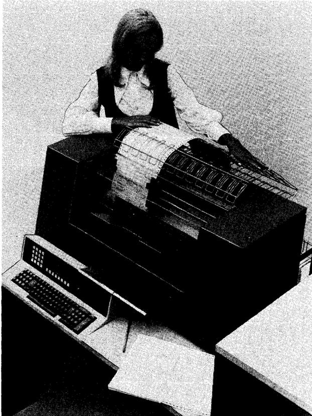
*This System/3 Model 6 is equipped with the wide-carriage 2222 Printer which enables it to handle ledger card processing. Cards up to 11 by 14 inches can be inserted into the feed slot (center).*
