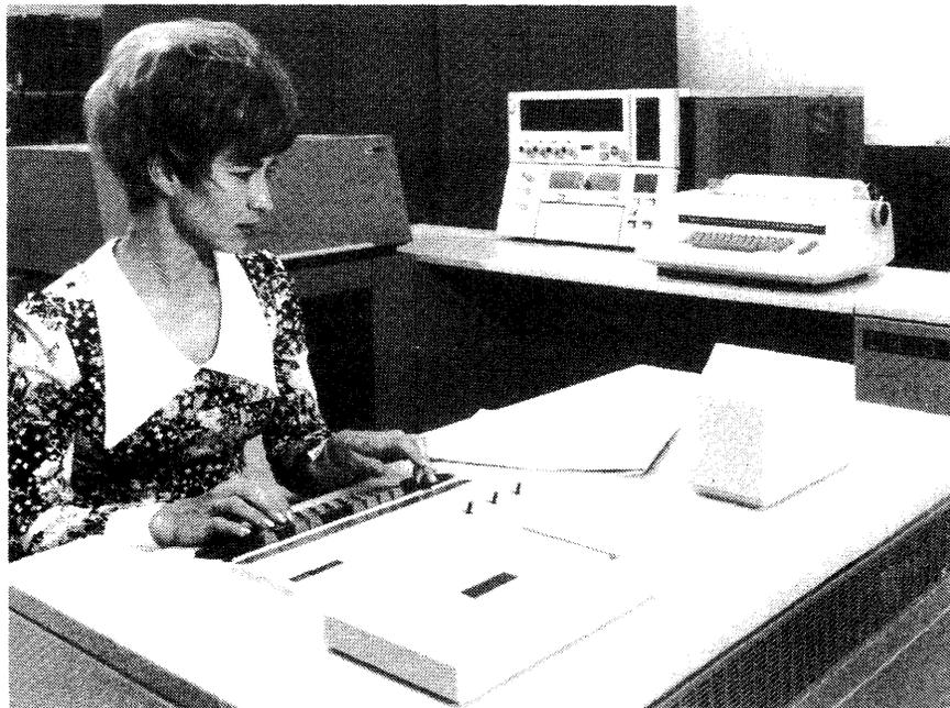
*The first cardless System/3 is the Model 8, introduced in September 1974. Its primary input device is the key-to-diskette 3741 Data Station shown in the foreground. The Model 8 is a disk-oriented system designed for efficient batch processing and communications functions.*
