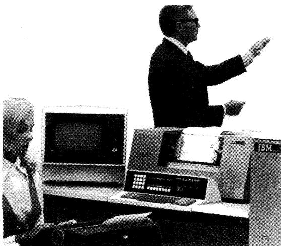
*The optional 2265 Display Station complements the basic 5213 Printer at right by serving as a high-speed output device for the transaction-oriented System/3 Model 6.*
