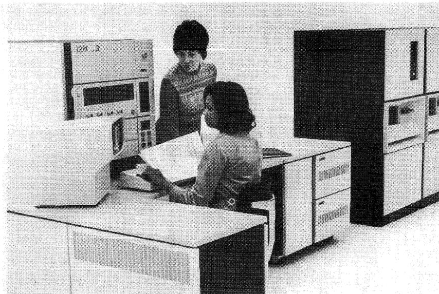
*The Model 15 is the most powerful and most expensive of the four versions of IBM's System/3. Thus, it's probably not for first-time computer users, but it provides the growth potential that many Model 10 users need. The Model 15 features an operator console with CRT display output, and can be equipped with up to 164 million bytes of on-line disk storage.*
