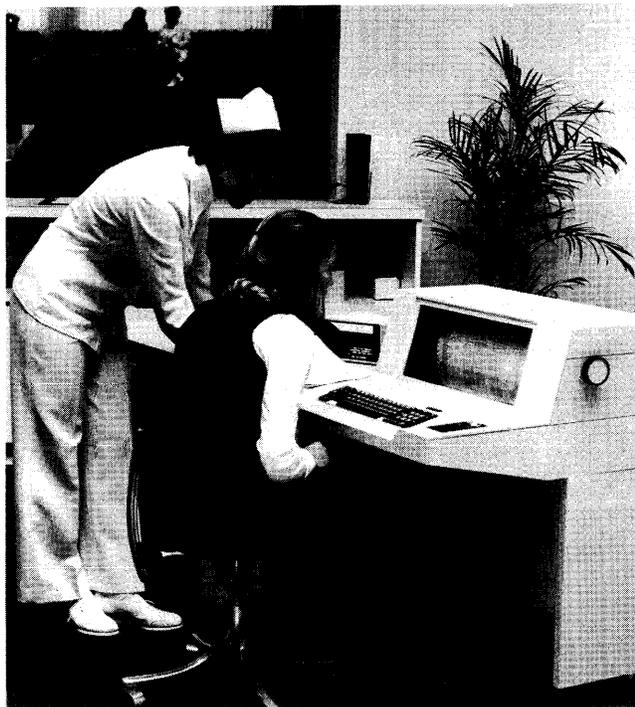
Shown here in a hospital application, the System/32 features a compact, integrated design that makes it suitable for a variety of office environments. The central processing unit, main memory, disk file, and diskette I/O unit are all housed in the desk-sized console to the left of the keyboard and printer. When equipped with the Hospital Financial Management System software, the System/32 is designed to meet the data processing needs of small hospitals with approximately 50 to 150 beds.
