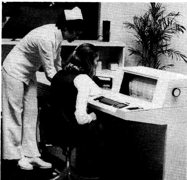
*Shown here in a hospital application, the System/32 features a compact, integrated design that makes it suitable for a variety of office environments. The central processing unit, main memory, disk file, and I/O unit are all housed in the desk-sized console to the left of the keyboard and printer.*
