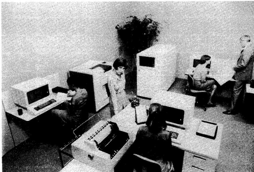
*This three-workstation System/34 configuration includes a 5340 System Unit with disk and diskette storage (center rear), a 5211 Line Printer (to left of System Unit), and three workstations mounted on customer-supplied furniture. Two of the workstations consist of 5251 CRT Display Stations, while the third (center foreground) includes both a 5251 Display and a 5256 Serial Printer. A System/34 can include up to eight workstations located up to 5000 feet away from the 5340 System Unit.*
