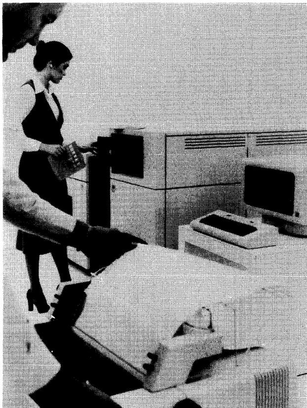
The System 34 is a member of the new wave of business computer systems packaged for use in standard office environments. Unlike the earlier IBM System 32, however, the System 34 offers a number of stand-alone peripheral devices, including both table-top and free-standing printers and a magnetic character reader.
