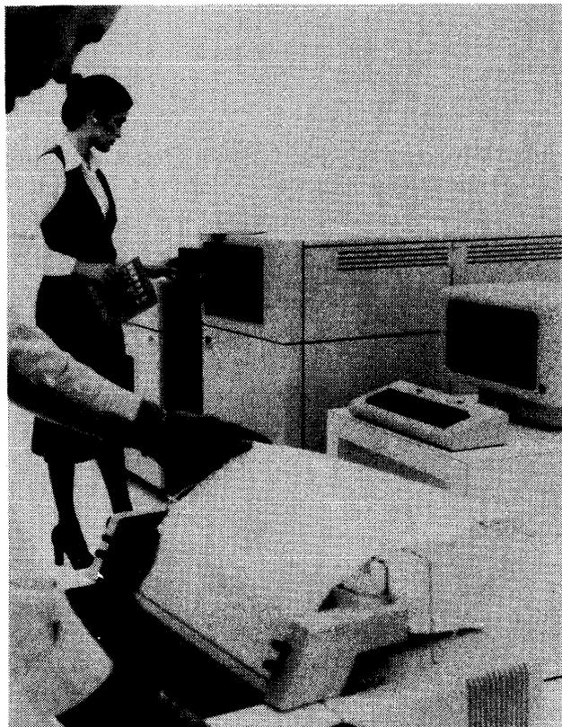
*The System/34 is a business computer system packaged for use in standard office environments. Unlike the earlier IBM System/32, however, the System/34 offers a number of stand-alone peripheral devices, including both table-top and free-standing printers and a magnetic character reader.*
