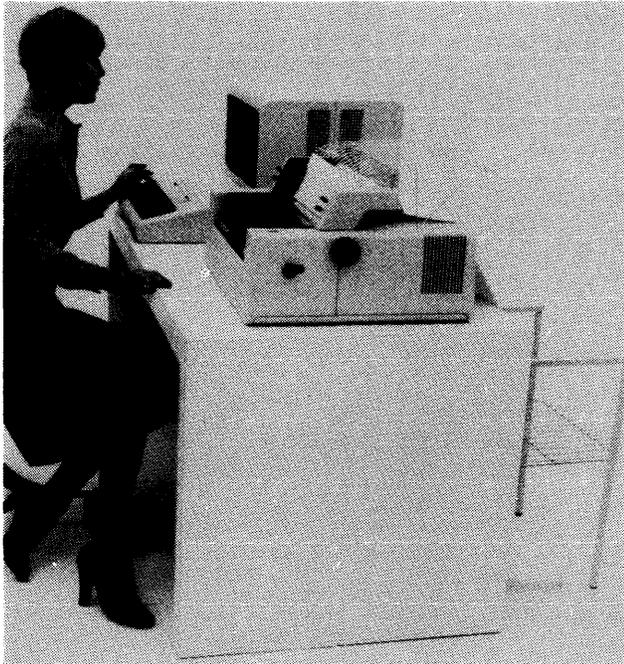
*The IBM 5250 Information Display System consists of the 5251 Display Station, Models 1, 2, 11, and 12; the 5252 Dual Display Station; and the 5256 Serial Printer, Models 1, 2, and 3. The 5250 components can be connected to the System/34 both locally (up to 16 workstations) and remotely (up to 64 workstations).*
