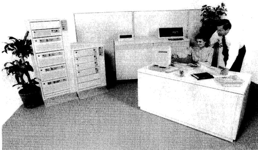
Six new models of IBM's System/38 offer users more flexibility, increased capacity, and improved performance at a lower cost, as well as enhanced connectivity with the IBM System/36. Two new advanced technology direct access storage devices, the IBM 9332 (left) and IBM 9335 (far left), provide System/38 users with more flexibility and options in system configuration, greater capacity (up to 13.6 gigabytes), and increased reliability.
