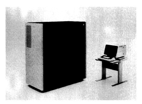
At the left is a picture of the 4381 processor and console which features from 4 to 16 megabytes of main memory, 4K to 32K bytes of buffer storage, and up to 12 I/O channels. It can utilize virtually all of the System/370 communications and peripheral equipment, including the high-performance 3380 Direct Access Storage Device. The 4381 supports the MVS/XA operating system as well as OS/VS1 and DOS/VSE.
