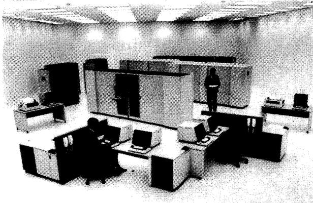
*IBM's family of large-scale computer systems, the 308X Series, currently has seven models available with memory capacities that range from 8 to 128 megabytes. The most powerful processor in the series, the 3084 QX, can operate as a tightly coupled four-processor system or as two independent dual-processor systems.*
