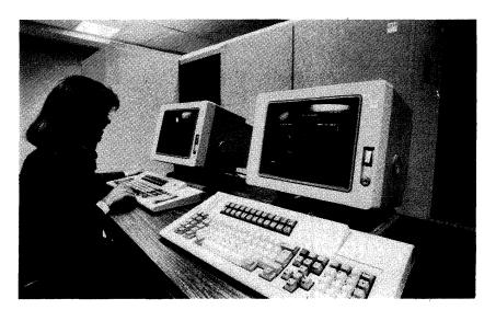
The IBM 3090 Model 200 dual processor, shown here, and the 3090 Model 400 four-way processor are IBM's newest top-of-the-line, large-scale computer systems. They feature Emitter Coupled Logic and Thermal Conduction Modules, and achieve a cycle time of 18.5 nanoseconds.
