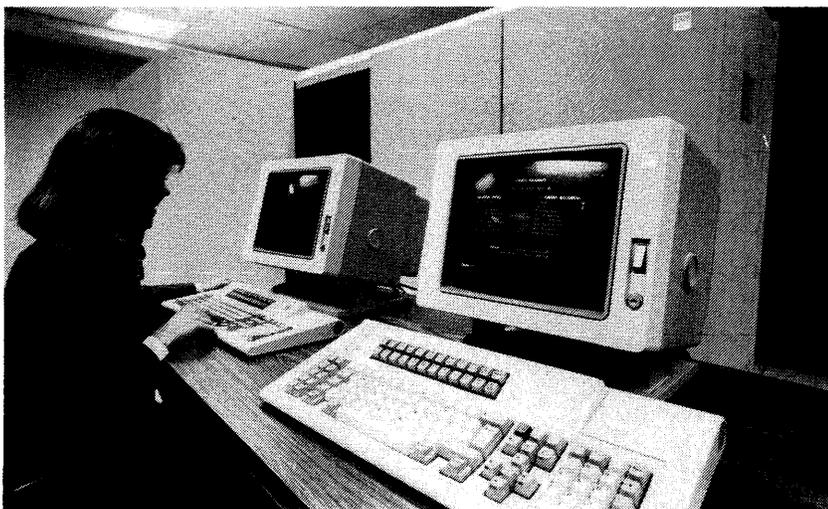
*The IBM 3090 Model 200 dual processor, shown here, and the 3090 Model 400 four-way processor are IBM's newest top-of-the-line, large-scale computer systems. They feature Emitter Coupled Logic and Thermal Conduction Modules, and achieve a cycle time of 18.5 nanoseconds.*
